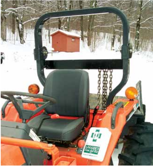
Figure 13.2. Every tractor and motor vehicle should have a first aid kit, and tractors should be equipped with a roll-over protective structure.
