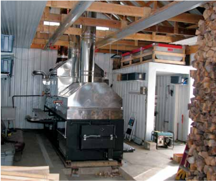
12.8. Many sugarmakers add wood storage onto the end of the sugarhouse nearest to the arch.
