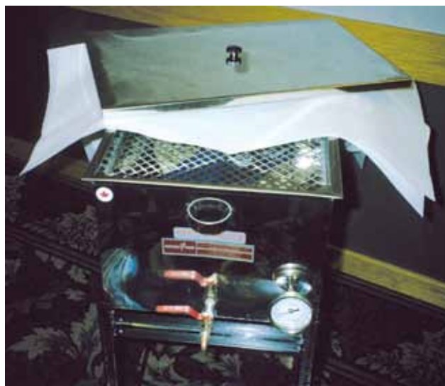
Figure 8.2. Flat gravity filter/bottling system showing filter sheet, paper prefilter (on top of “felt” filter), and supporting screen.
