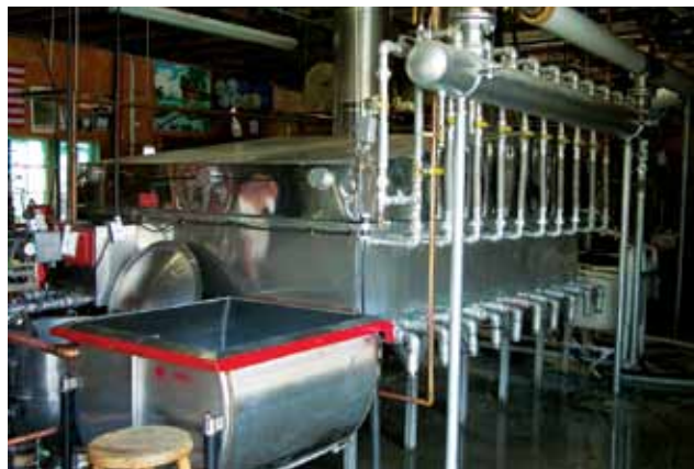
Figure 7.18. Five natural gas burners in front wall of arch.
