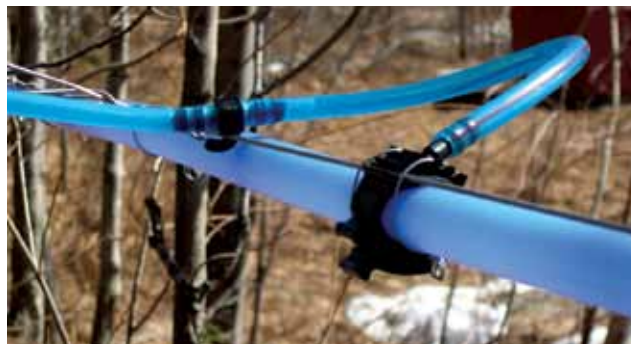
Figure 6.22. A saddle-type or multi-fitting is installed by drilling a small hole in the mainline and placing the fitting (right in picture) over the hole. The hook connector (left in the picture) hooks onto the mainline support wire and relieves the tension on the fitting.
