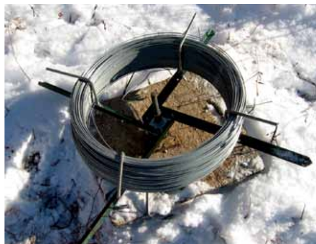
Figure 6.14. A wire spooler is a useful tool for avoiding kinks in wire when pulling it through the sugarbush.
