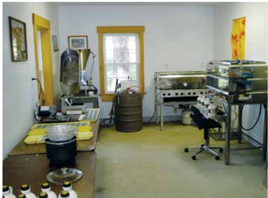
Figure 9.1. A spacious, clean, ordered, well-equipped area is desirable for making maple products. Equipment visible includes container and basket for crystal coating candy (left front), soft sugar candy machine with molds (left middle), maple cream machine (left rear), syrup barrel (rear center), propane-fired syrup reheating pan (right rear), canister pressure filter (right middle on floor), and syrup canning equipment (right front). (Ober)
