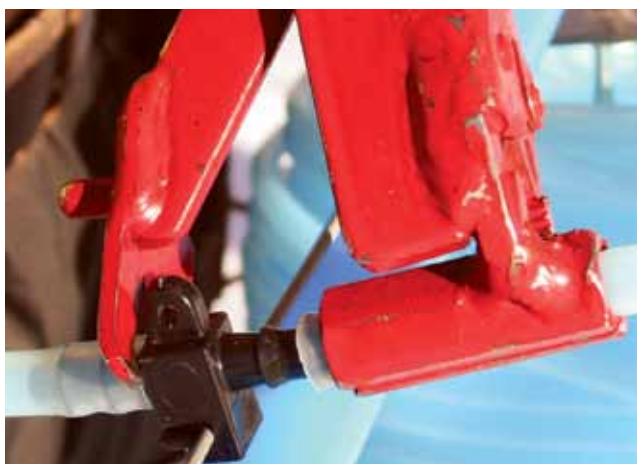
Figure 6.24. Double tubing tool (top) being used to cut in dropline; one-hand tubing tool (bottom) being used to install hook connector (see Figure 6.22).
