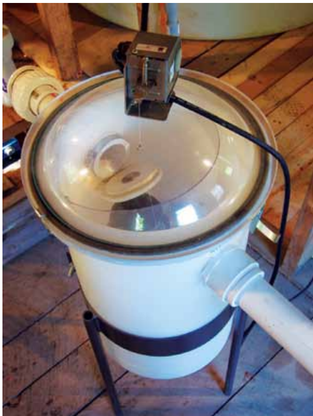
Figure 6.33. One form of moisture trap. A moisture trap should be installed between the vacuum pump and the extractor to reduce the potential for moisture damage to the pump.
