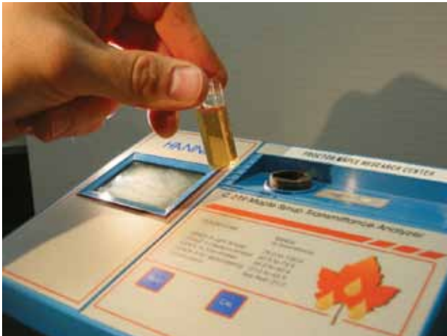
Figure 8.11. Relatively inexpensive spectrophotometer for determining the color of maple syrup based on light transmission.
