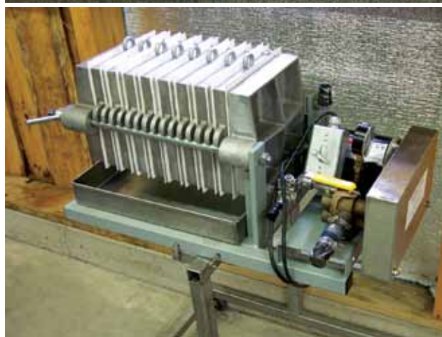
Figure 8.3. Canister (top) and plate (bottom) pressure filters.
