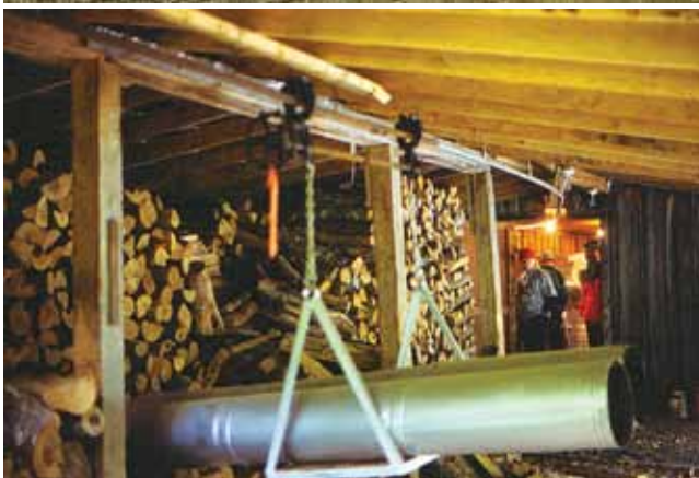
Figure 12.9. Sugarmakers have found many inventive ways to transport firewood, including ground rails, pallets, and a carriage suspended from an overhead rail.
