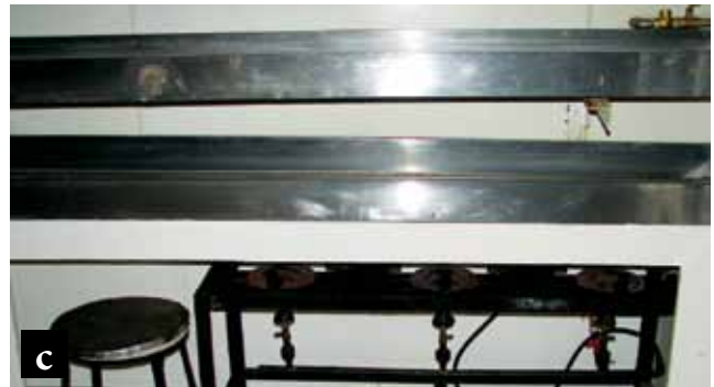
Figure 9.3. A water bath provides the rapid cooling required for several maple products during processing. Depending on the size of the batches and the frequency they are made, a small tub (a), a stainless sink (b), or a trough specifically designed as a cooling bath (c) might be most appropriate. (Douglass, Freeman, Ober)
