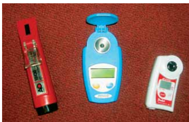
Figure 8.6. Optical refractometer (left) and digital refractometers (center and right).
