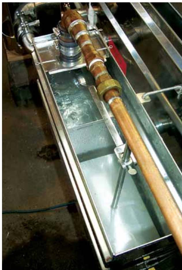
Figure 7.5 Regulator box on the side of the flue pan, which controls the flow of sap into the flue pan. In this regulator box, sap flow into the flue pan is controlled by a float valve.
