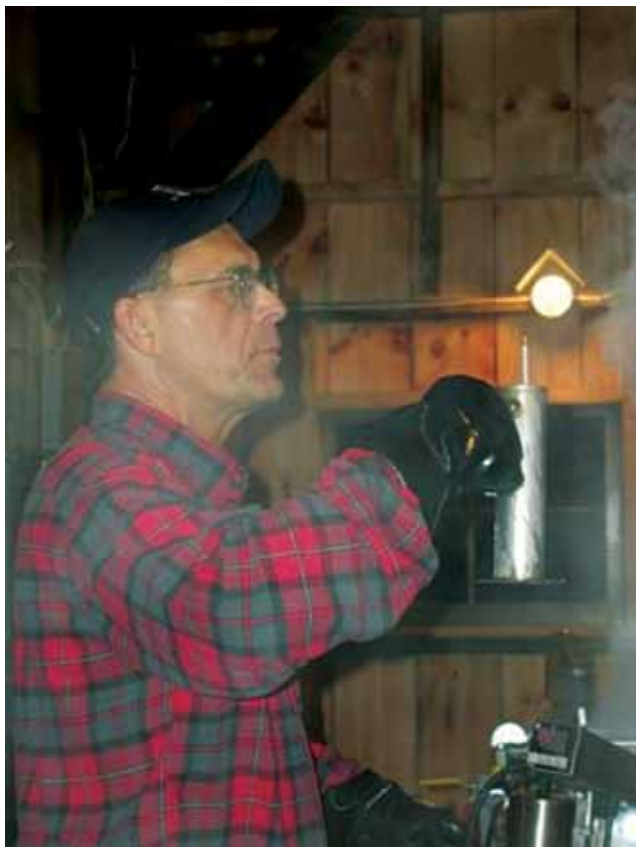
Figure 7.24. Hot testing with a hydrometer to determine syrup density. (Girard)
