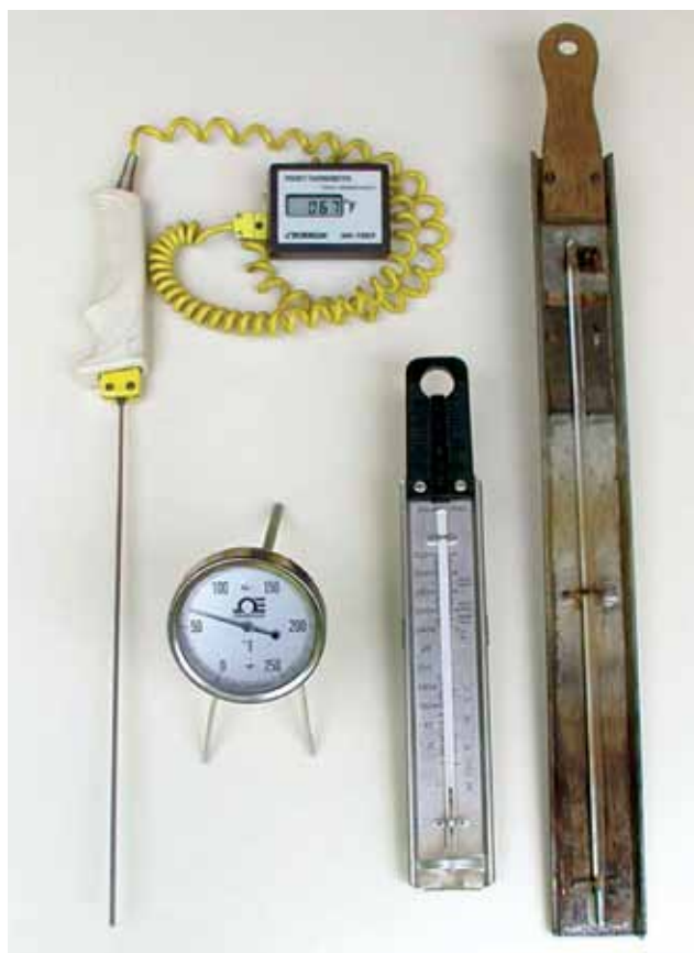
Figure 9.2. Digital, dial, or stem-type candy thermometers can all successfully be used to make maple confections.
