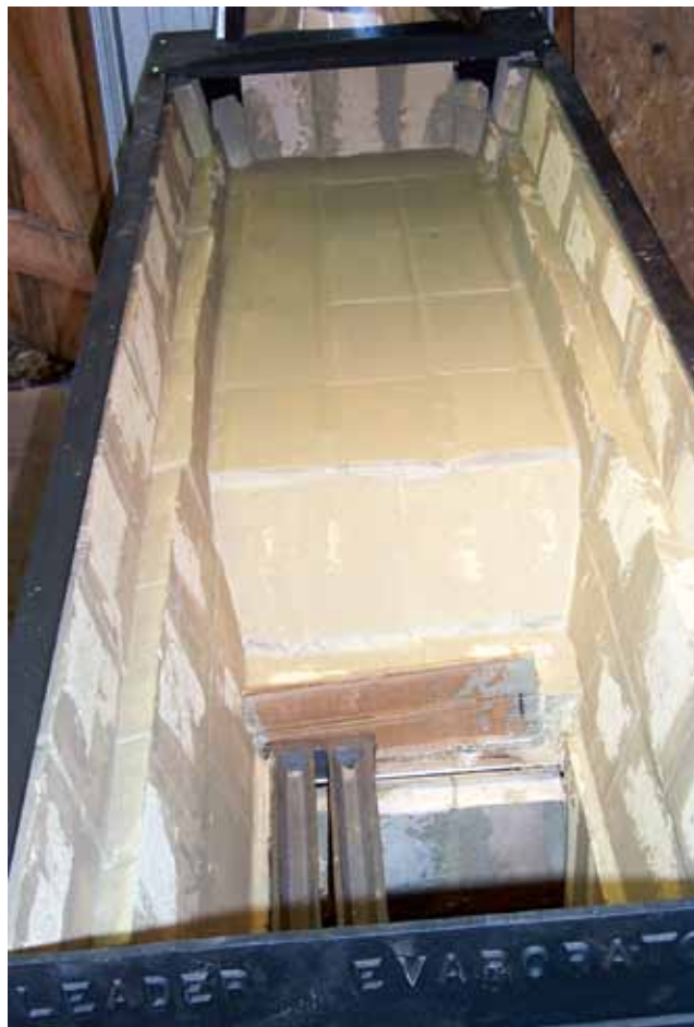
Figure 7.12. Wood-burning evaporators must be lined with firebrick next to the fire to avoid damage to the insulation.
