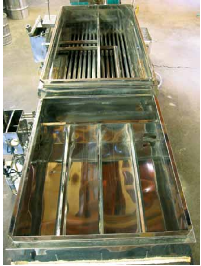
Figure 7.6. Evaporator with a raised flue sap pan and two cross flow syrup pans (left) and an evaporator with a drop flue sap pan and a reverse flow syrup pan (right). In regard to the sap pans, note that the top of the raised flue sap pan sits somewhat higher relative to the syrup pan than the drop flue sap pan. With respect to the syrup pans, note that this particular reverse flow pan has four parallel channels and a fifth at right angle (nearest the sap pan) that allows the flow to be reversed without changing the draw-off side. Many reverse flow pans do not have the right angle channel but only the parallel channels, and the draw-off side must be switched when the flow is reversed.
