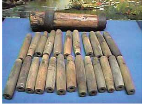
Figure 2.1. Primitive spouts were small stem sections of sumac or elder that were hollowed out by removing the central core or pith tissue. (Girard)
