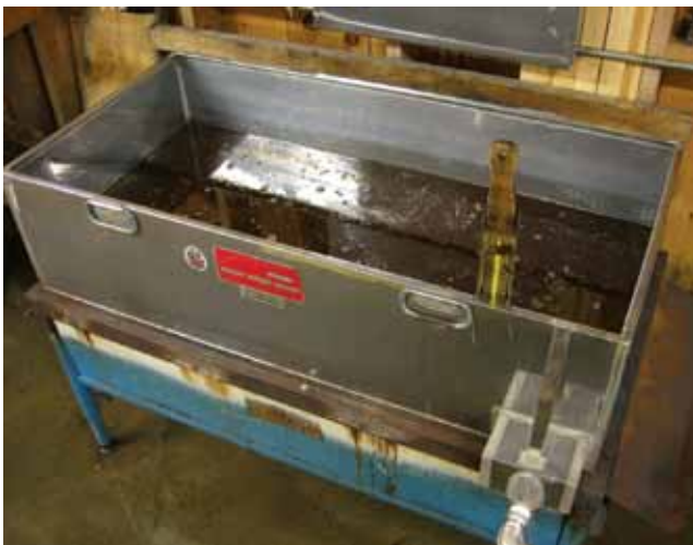
Figure 7.26. A gas heated finishing pan.
