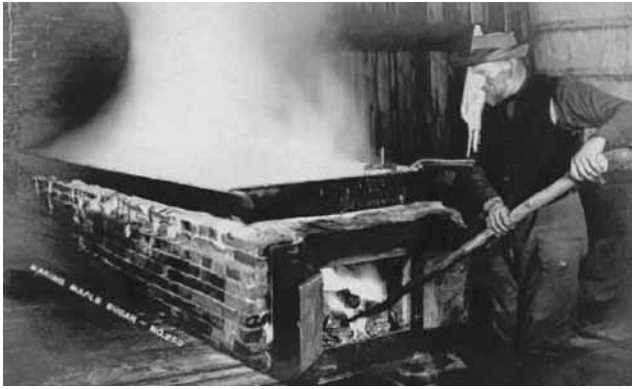
Figure 2.9. Sometime in the mid-1800s the flat-bottomed pan mounted on an arch developed for concentrating sap was introduced. (Girard)
