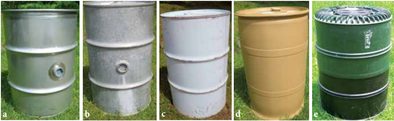
Figure 8.14. The most common type of bulk containers used in the maple industry today include: stainless (a), galvanized (b), epoxy (c), and food-grade plastic (d). A fifth container, plastic with a food-grade, replaceable liner, is also available (e). Stainless containers or those made of food-grade plastic are recommended for maintaining the quality of maple syrup.
