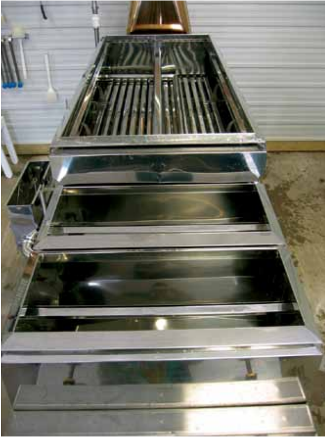
Figure 7.6. Evaporator with a raised flue sap pan and two cross flow syrup pans (left) and an evaporator with a drop flue sap pan and a reverse flow syrup pan (right). In regard to the sap pans, note that the top of the raised flue sap pan sits somewhat higher relative to the syrup pan than the drop flue sap pan. With respect to the syrup pans, note that this particular reverse flow pan has four parallel channels and a fifth at right angle (nearest the sap pan) that allows the flow to be reversed without changing the draw-off side. Many reverse flow pans do not have the right angle channel but only the parallel channels, and the draw-off side must be switched when the flow is reversed.
