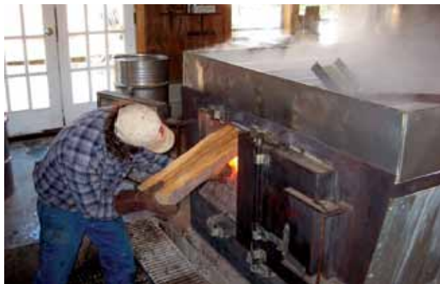
Figure 7.20. Alternating door method of firing wood-burning evaporator.
