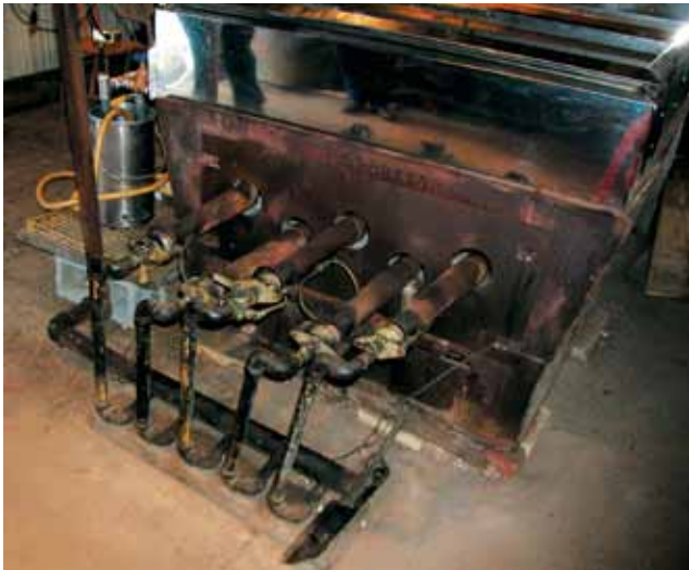
Figure 7.18. Five natural gas burners in front wall of arch.
