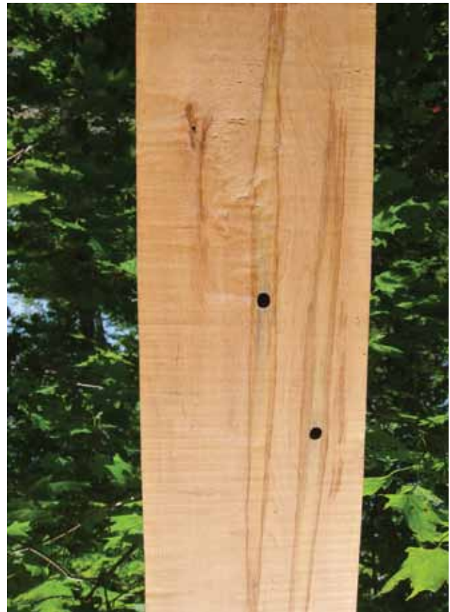
Figure 6.6. The zone of discoloration from a taphole (or other wound) can extend 12 or more inches above and below.
