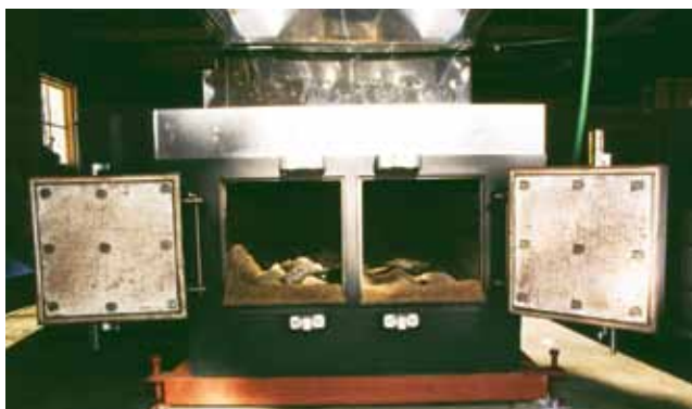
Figure 7.14. Insulated arch doors dramatically increase the efficiency of a wood-burning evaporator.
