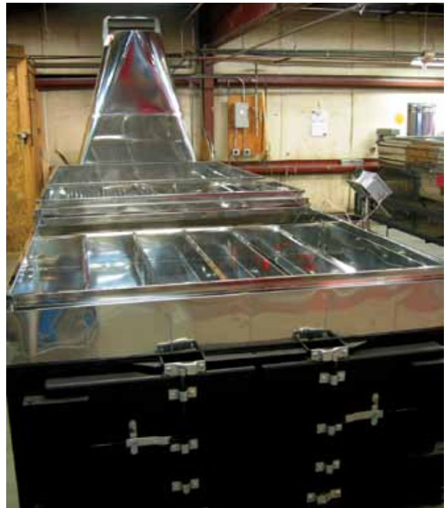
Figure 7.4. Older, basic evaporator (top) and more modern evaporator (bottom) showing arch, front (syrup) pan with partitions, and back (sap) pan with flues.
