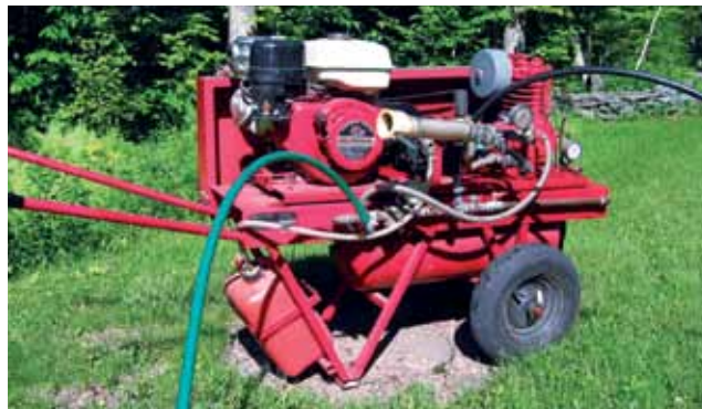
Figure 6.30. Gasoline powered air/water pressure tubing washer. Essentially a gasoline engine powered air compressor and a water pump (hidden to right of gasoline engine) along with appropriate gauges, valves, and supporting hardware to provide a pressurized mix of air and water to the black line on the right.
