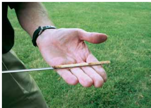
Figure 5.7. An increment borer (in use, top) is used to extract a core of wood from the trunk of a tree that shows the tree rings. If the core is taken to the center of the tree, the tree's age can be determined by counting the annual rings. Shorter cores are used to determine the tree's growth rate over some time period, usually the past 5 or 10 years, or to look for a slowing of the tree's growth rate, a possible indicator of increased competition from surrounding trees.
