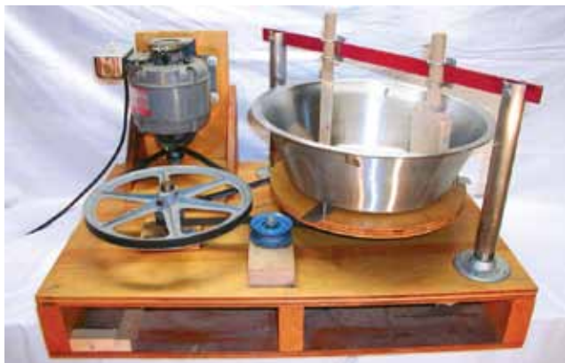
Figure 9.5. It is possible to construct your own maple cream machine from readily available materials.
