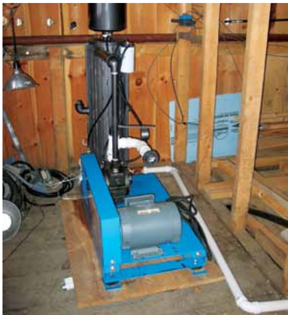
Figure 6.31. An oil-cooled vacuum pump appropriate for use with a tubing system.
