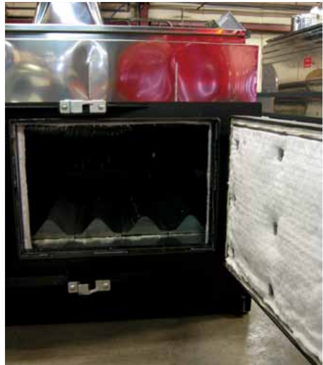
Figure 7.16. Modern, efficient wood-burning arch includes such features as insulated doors, positive door latch to prevent air leakage, double wall arch with insulation between walls, and forced draft with air injecting grates.
