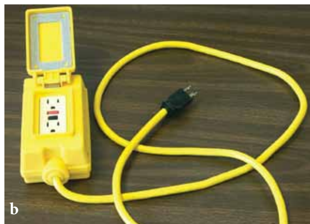
Figure 13.8. Permanently installed (a) or portable (b) ground fault circuit interrupters (GFCI) should be used to protect all circuits in the sugarcane house.
