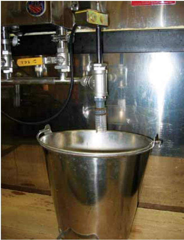
Figure 7.25. An automatic draw-off unit monitors the temperature in the syrup pan and automatically opens a solenoid valve to draw-off sap or syrup when the desired density is achieved.
