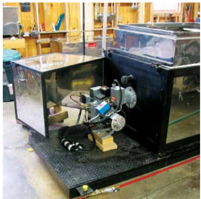
Figure 7.17. Modern oil burner used to fire maple evaporator.
