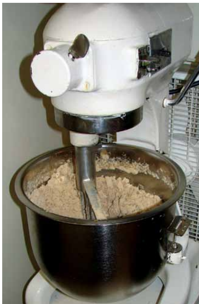
Figure 9.7. The difficult job of stirring maple sugar can be made a lot easier with a heavy-duty mixer. (Freeman)
