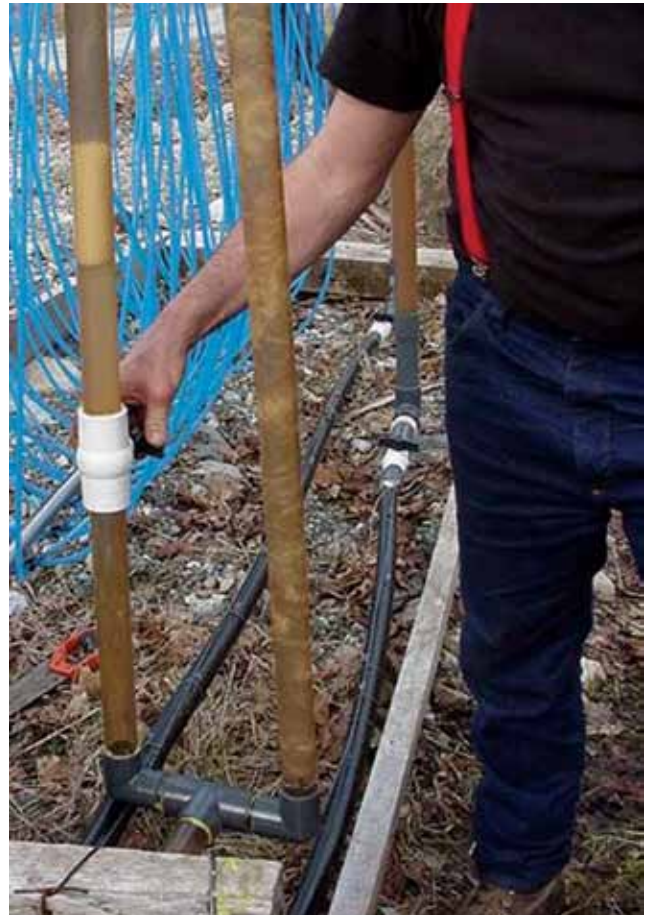
Figure 6.28. Pipe sap ladder in foreground. Producer has hand on shut-off valve that can be used to convert two pipe sap ladder to a single pipe sap ladder.
