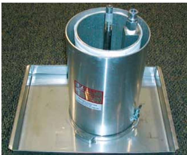
Figure 8.5. Inner and outer canister of canister pressure filter showing filter cloth around inner canister.
