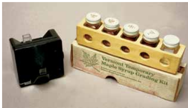
Figure 8.9. Permanent glass standard grading kits, such as the Lovibond (upper left) and the USDA kit (Figure 8.10), and temporary glycerine grading kits, such as the Vermont temporary kit (upper right), are available for color grading maple syrup.
