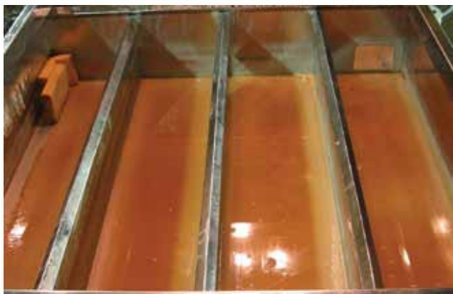
Figure 7.21. Heavy sugar sand build-up.
