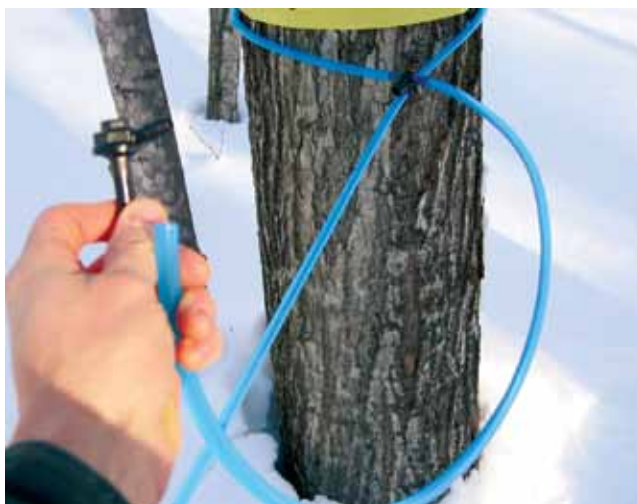
Figure 6.23. One of a variety of fittings designed to anchor the end of a lateral line. This particular end ring fitting accommodates a dropline (in the producer's hand).
