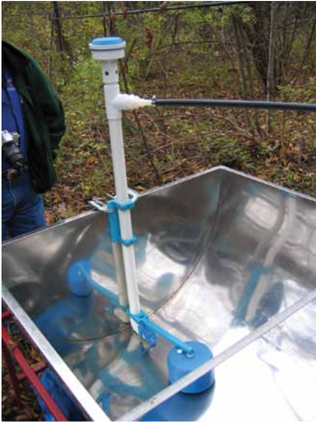
Figure 6.27. A mechanical vacuum extractor can be used to transfer sap collected from taps situated at an elevation lower than a collection or storage tank.
