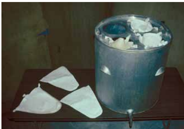
Figure 8.1. Felt-hat filter system, showing filter tank, paper prefilter (left top), and “felt” cone filters.
