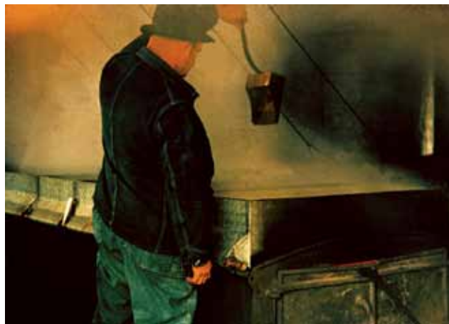
Figure 7.22. Determining finished syrup using the apron test.
