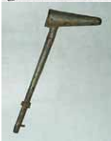
Figure 2.5. Early gooseneck tubing system. (Girard)
