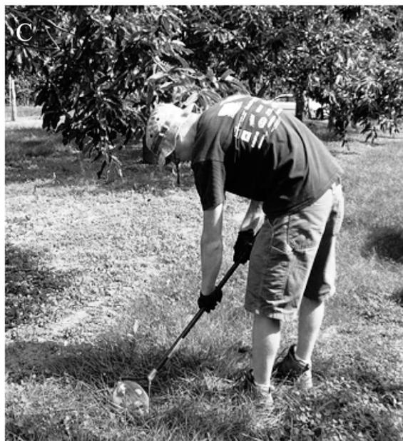
**Fig. 1.** Harvest equipment evaluated for harvesting chinese chestnuts: (A) pasture vacuum (Paddock Vac; Greystone Vacuums, Monroe, WA), (B) modified pasture vacuum (Maxi Vac, Greystone Vacuums) with raised collection tank and open-weave metal shelf, and (C) manual nut-harvesting tool (Nut Wizard, Holt’s Nut Wizard, Douglas, GA).
